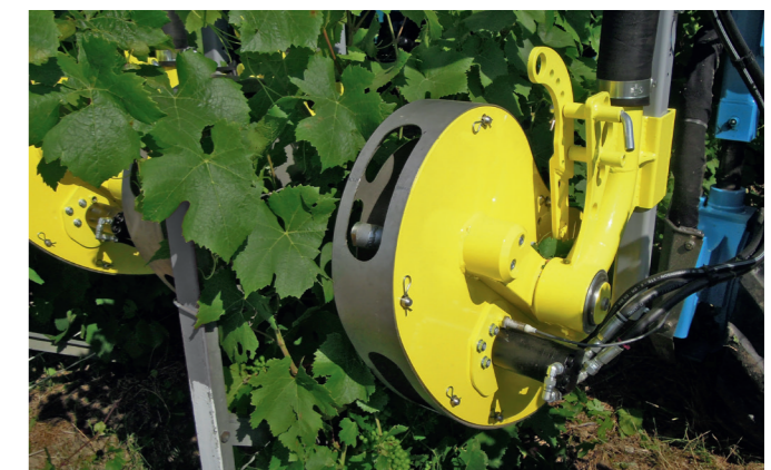
▲ Air distributors drive by motors and drained. Integrated electronic speed sensor.
