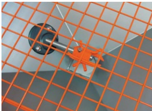
Standard filtering grids and mixer with ultra-slow rotation
